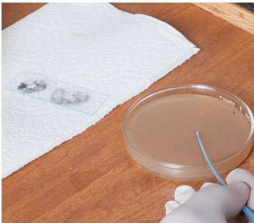
Transfer spores from a slide or piece of foil to the petri dish; in this photo I'm using an inoculation loop. Spread spores across the middle of the dish in an "S" pattern.
