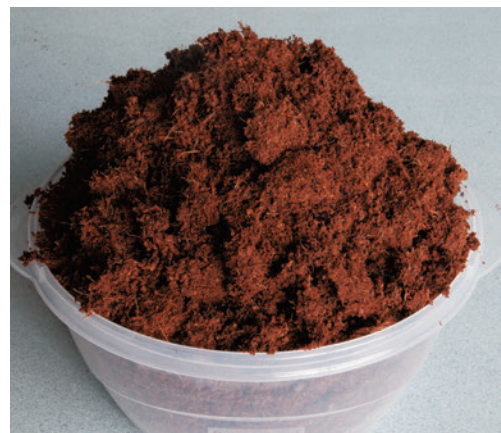
Coir is commonly sold in compressed bricks. Before it can be used, it must be soaked in water.
